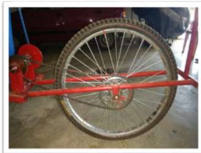
Figure 5: Assembly of Wheel, Chain & Sprocket
