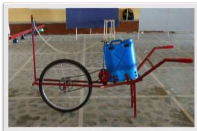
Figure 6: Working Model Of Multi Nozzle Wheel Spray Pump
